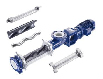
Among their many uses, progressing cavity pumps are chosen for the pumping of sludges, polymers, and chemicals in water/wastewater treatment plants. Over the pump's life, typical maintenance may require the replacement of the stator and/or rotor. The innovative seepex Smart Conveying Technology (SCT) design greatly reduces maintenance time and cost to replace these parts.
